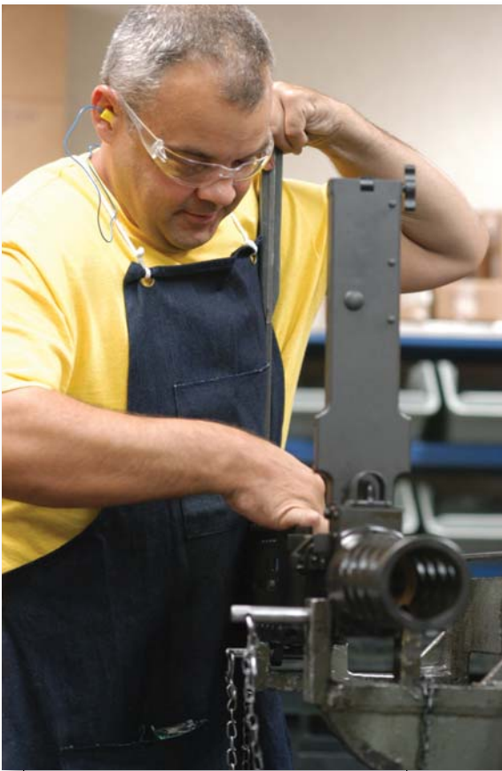
Above: Jeffrey Bonner works in the Anniston Army Depot's small-arms repair shop. Here he is putting an M-2 .50-caliber machine gun back together.
