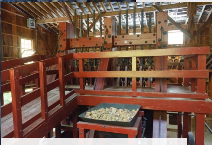
Top Left: Entrance to the Reed Gold Mine State Historic Site. Above: The 10-stamp mill is a machine that crushes material by pounding rather than grinding for extraction of the metallic ore. Right: A mine cart used for moving ore and materials.
