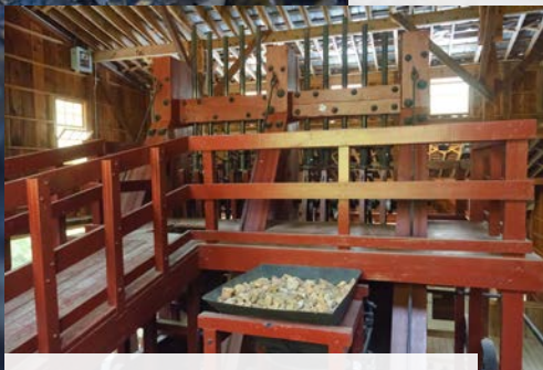
Top Left: Entrance to the Reed Gold Mine State Historic Site. Above: The 10-stamp mill is a machine that crushes material by pounding rather than grinding for extraction of the metallic ore. Right: A mine cart used for moving ore and materials.
